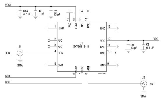
Figure 3. SKY66113-11 Reference Design Schematic
