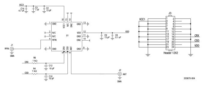
Figure 4. SKY66113-11 Evaluation Board Schematic Diagram
