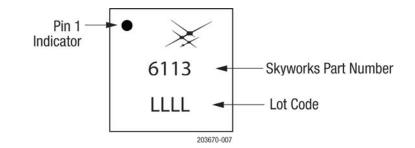
Figure 7. SKY66113-11 Typical Part Marking (Top View)
